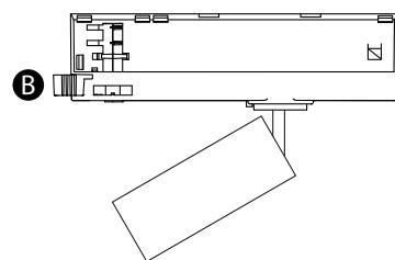
Rotate adaptor lock **B** clockwise to connect the adaptor to the neutral circuit.
