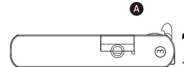
Circuit 1: Rotate the knob **A** clockwise from the starting position OFF, to connect circuit 3.
