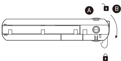
To mount the track adaptor into the track system, first check that the selector knob **A** is at OFF position and the adaptor lock **B** is disengaged.
