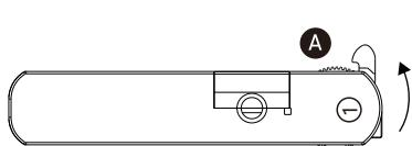
Circuit 1: Rotate the knob **A** clockwise from the starting position OFF, to connect circuit 1.
