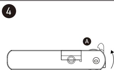
Rotate selector knob **A** to the position of desired circuit.
