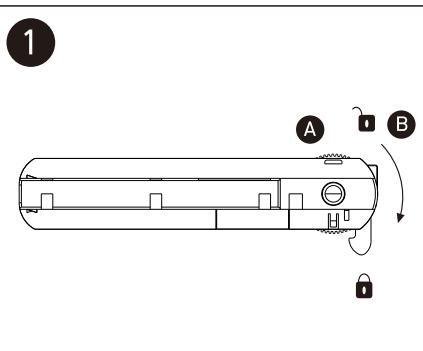
To mount the track adaptor into the track system, first check that the selector knob **A** is at OFF position and the adaptor lock **B** is disengaged.
