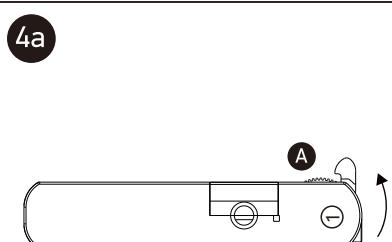
**Circuit 1:** Rotate the knob **A** clockwise from the starting position OFF, to connect circuit 1.
