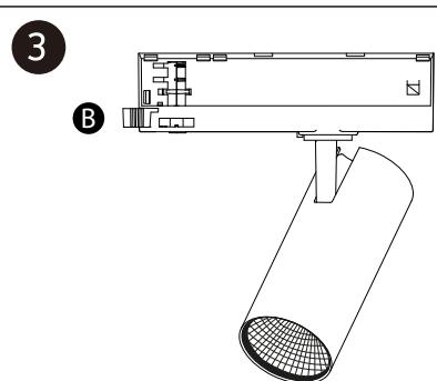
Rotate adaptor lock **B** clockwise to connect the adaptor to the neutral circuit.
