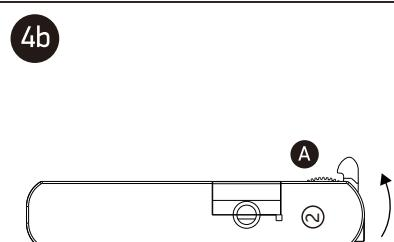
**Circuit 2:** Rotate the knob **A** counter-clockwise from the starting position OFF, to connect circuit 2.
